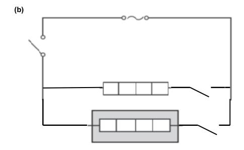
switches in both heater branches (can be either side of heater);
